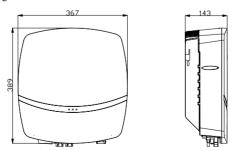
Figure 3.3 Dimensions of R5-3K/3.6K/4K/5K/6K-S2
