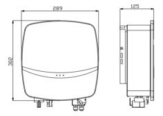
Figure 3.2 Dimensions of R5-0.7K/1K/1.5K/2K/2.5K/3K-S1
