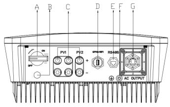
Figure 5.3 Electrical interface of R5-7K/8K-S2
