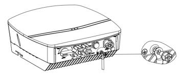
Fig. 5.4 Inverter ground protection
