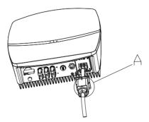
Fig. 5.9 Connecting the cable
