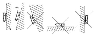
Figure 4.1 Mounting method
