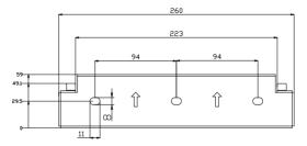
Figure 4.3 Dimensions of rear panel of R5-0.7K/1K/1.5K/2K/2.5K/3K-S1
