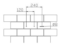
Figure 4.7 Drill holes' dimensions of R5-3K/3.6K/4K/5K/6K/7K/8K-S2
