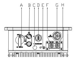
Figure 5.1 Electrical interface of R5-0.7K/1K/1.5K/2K/2.5K/3K-S1
